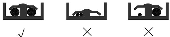
Use the specified electric wire. Connect the wire securely to the terminal. Lock the wire down without applying excessive force to the terminal. (Tightening torque:  $1.31\text{N}\cdot\text{m} \pm 10\%$ ).
