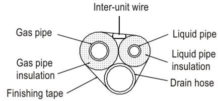
3) Finally, insulate as shown in the figure below.
