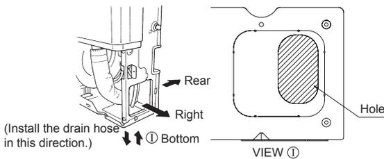
For direction ① (Bottom), bore the oval hole shown in the above figure. The drain hose can be connected to either the left or right side.
