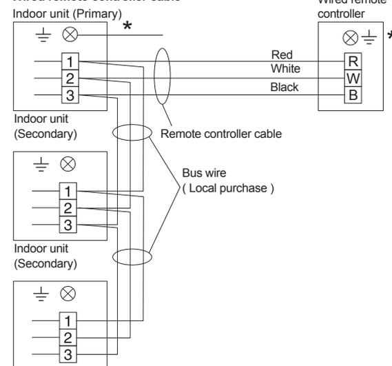
\*Earth (Ground) the remote controller if it has a earth (ground) line.
