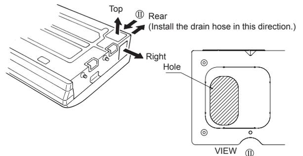
For direction ① (Rear), bore the oval hole shown in the above figure.
