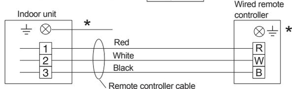
\*Earth (Ground) the remote controller if it has a earth ground) line.
