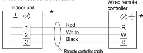
\*Earth (Ground) the remote controller if it has a earth ground) line.
