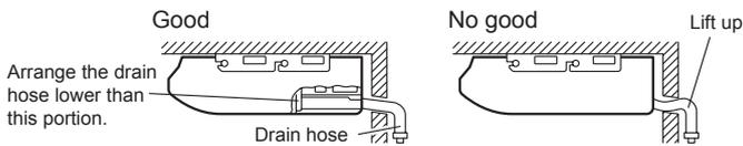
When drain hose is arranged backward. Secure the drain hose with the VT wire.
