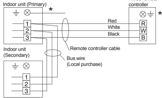
\*Earth (Ground) the remote controller if it has a earth (ground) line.
