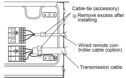
(5) Install the electrical component box in the original position after securing the cover.
