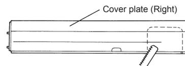
(2) Join the cover plates (right) and mount with the screw (ø4 × 10).
