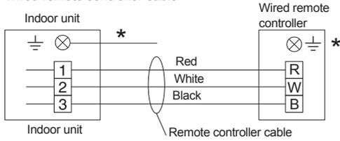
\*Earth (Ground) the remote controller if it has a earth (ground) line.
