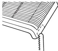
(2) Insert the hinges on the bottom of the intake grille into the holes in the base assembly. Then mount the arms to the 3 areas on the top of the intake grille.
