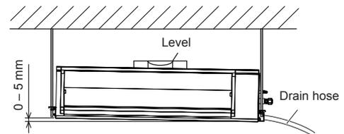
Give a slight tilt to the side to which the drain hose is connected. The tilt should be in the range of 0 mm to 5 mm.
