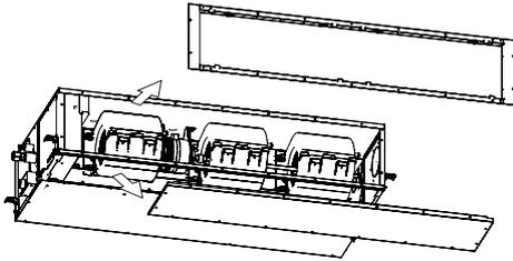
For the bottom air intake, position (1) the intake grille, and (2) the service panel, as shown in the following figure. (The factory setting is back air intake.)
