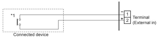
\*1: The switch can be used on the following condition: DC 12 V to 24 V, 1 mA to 15 mA.
