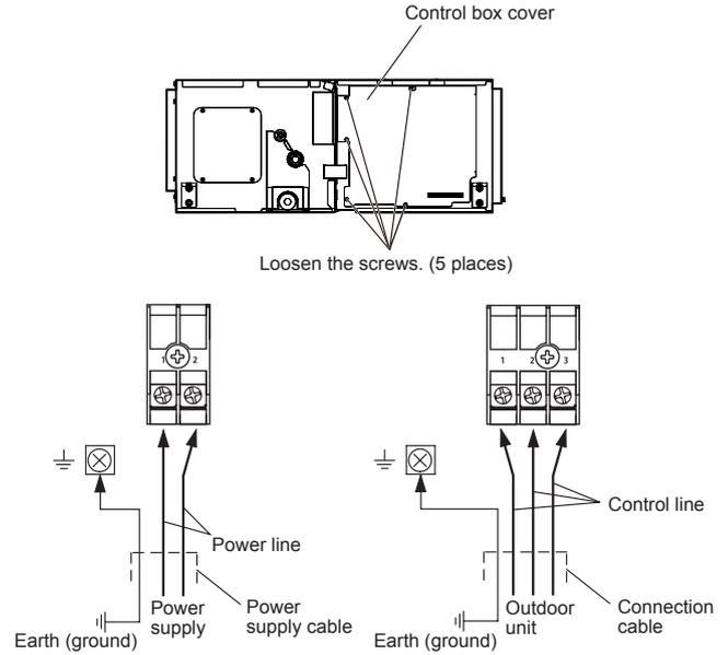
NOTES: Be sure to connect both the power supply and connection cables accordingly. If both cables are not connected, the air conditioner will not function properly.
