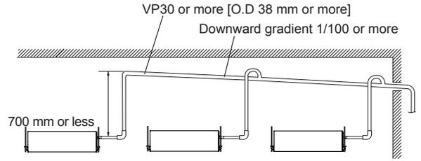
4. 4. 3. When drain pump is not used (Natural drainage)
