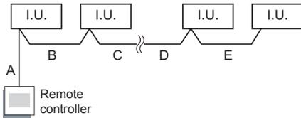
A, B, C, D, E : Remote controller cable. (Refer to "3.3. Electrical requirement")
