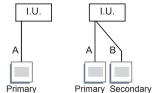
A, B : Remote controller cable. (Refer to "3.3. Electrical requirement")
