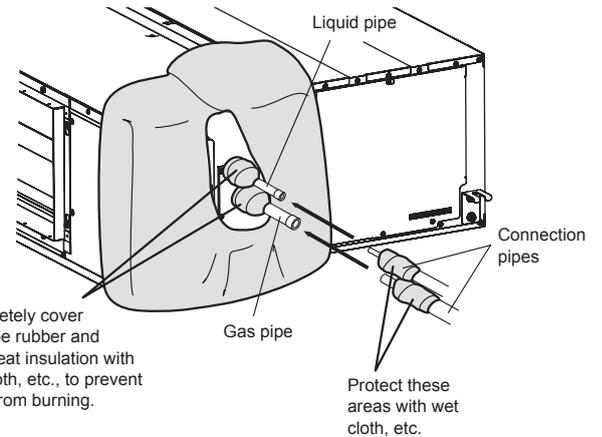
Completely cover the pipe rubber and pipe heat insulation with wet cloth, etc., to prevent them from burning.
