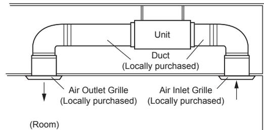
When connecting the duct, perform duct-insulation appropriate for the installing environment. Inappropriate insulation work may cause condensation on the surface of the insulating material, and may lead to condensation dripping.
