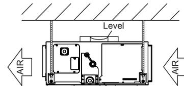
Base horizontal direction leveling on top of the unit.
