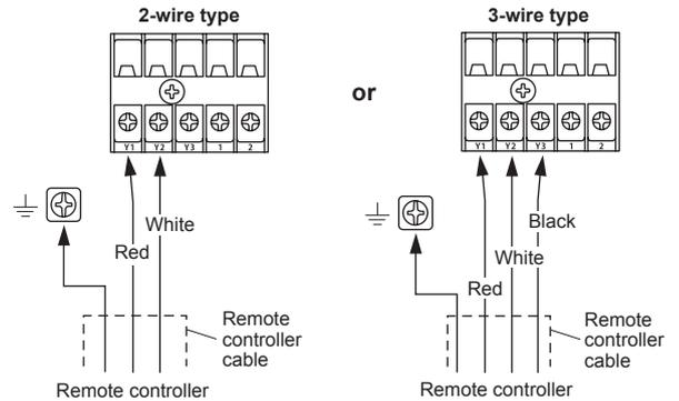
\*Earth (Ground) the remote controller if it has a earth (ground) wire.
