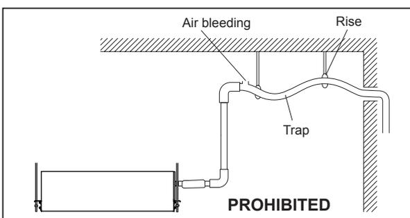
Observe the following procedures to construct centralized drain pipe fittings.
