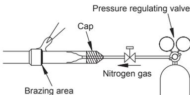
If a pipe is brazed without applying nitrogen gas, it will create an oxidation film. This can degrade performance or damage the parts in the unit (such as the compressor or valves).
