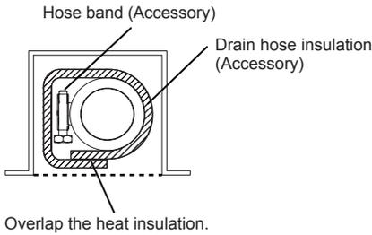
4. 4. 2. When drain pump is used (Option is necessary for 72/90 type)
