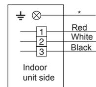
\*Ground the remote controller if it has a earth (ground) wire.
