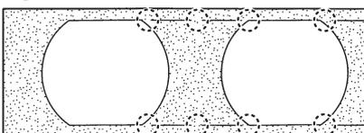
(2) Turn up the insulation around the points to be cut according to the outlet port shape working points so that the insulation does not stick out at the **CUT** part.
