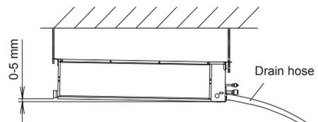
Give a slight tilt to the side to which the drain hose is connected.
