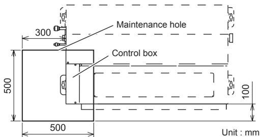
It shall be possible to install and remove the control box, fan units and filter.
