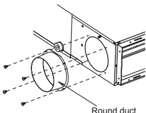
(3) Connect the duct to the round flange.
