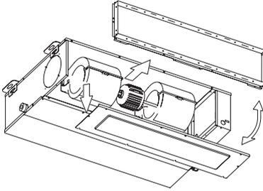
For the bottom air intake, follow the procedure of ①→② for installation. (The factory setting is back air intake.)
