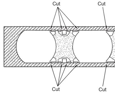
(3) Cut with nippers and remove the sheet metal.
