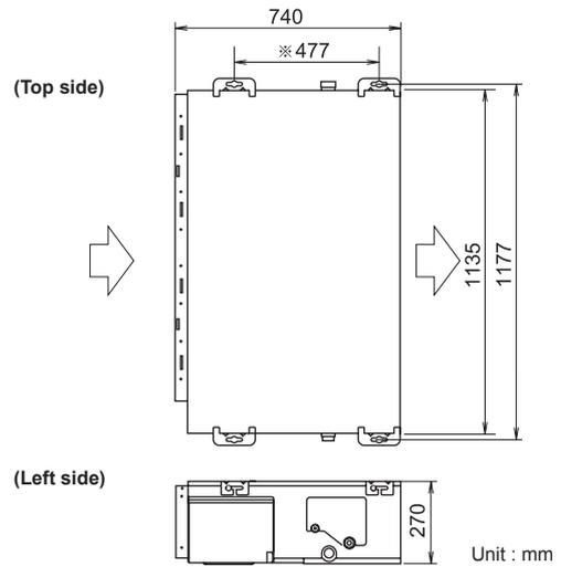
The distance of \* is adjustable according to the place of the hanging bolts.
