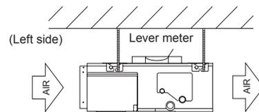
Base horizontal direction leveling on top of the unit.
