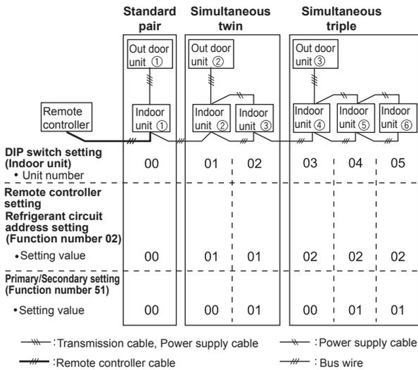
Make sure that the indoor unit with the unit number 00 is connected to the outdoor unit using a transmission cable.
