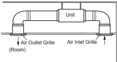
When connecting the duct, perform duct-insulation that is appropriate for the installing environment.
